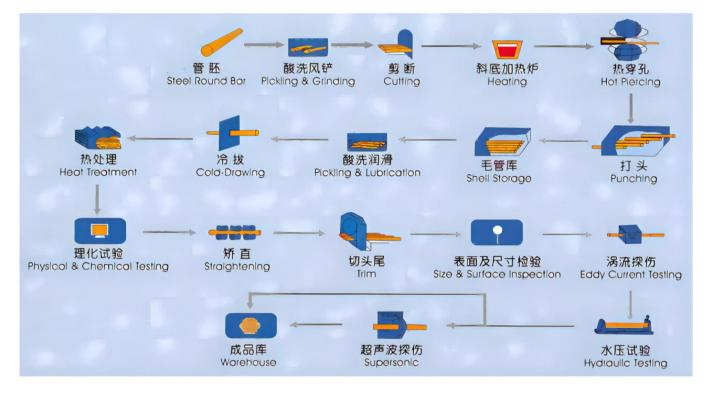
Hot-finished tubes are manufactured at high temperatures and have better toughness but rougher surfaces and lower dimensional accuracy; whereas cold-drawn tubes are manufactured by plastic deformation at room temperature and have higher strength, smoother surfaces, and more precise dimensional control, making them suitable for applications that require higher precision and performance.
